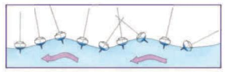
Vessels may experience resonant rolling if encountering a series of fairly regular beam waves. The waves do not have to be especially large, but may just have a period similar to the natural rolling period of the boat. Due to the damping effect of wind in the sails, this is generally of less concern to vessels under full sail.
