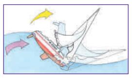
trough of the wave while the stern is being lifted by wind and sea. The stern is then lifted OVER the bows!
