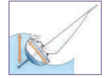
4 Multihulls and form-stable monohulls reach maximum stability at a relatively small angle of heel (typically 10° to 15°) and very seldom have sufficient righting moment at 90° heel to overcome the wind forces on the bridge-deck structure. Virtually all multihulls and form-stable monohulls are therefore capable of being capsized by wind action alone if too much sail is carried.
