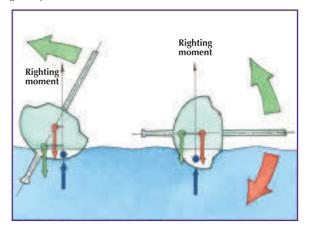
excessive weight, or by raising the point of suspension too high. A very slow rolling motion is a sign that this condition may be being reached.
