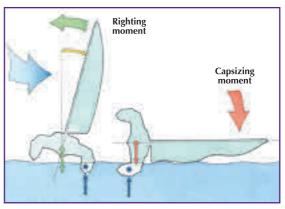
It is therefore vital that the amount of sail carried is not sufficient to cause capsize, even in a gust, which may cause a doubling of wind heeling moment.
